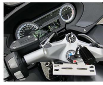
The new R 1200 RT-P raises the standard for electrical power management while providing fast and efficient connection of police equipment. The BCa (Body Controller authority) controls all special authority circuit outputs and charging of the auxiliary battery. There is no need for fuses, the BCa monitors and protects outputs, controlling circuits for all police accessories:
